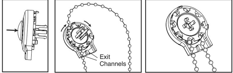
Release the center post which will trap the loop. Be sure the control cord/chain exits the channels at the narrow end as shown.
