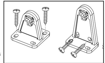
On inside mount shades the Tension Device may be mounted to the window sill, or side window frame or when the treatment spans beyond the window frame it may be mounted to the wall.
