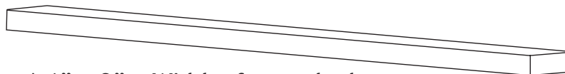
A 1" x 2" x Width of your shade Wood Board for a 15LB System or A 1" x 3" x Width of your shade Wood Board for a 30LB System
